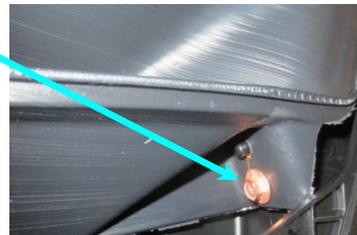
1.2 Disconnect the vehicle harness data link connector from the Smart Data Link module for the harness installation (Ignition must be off including all accessories off.)
